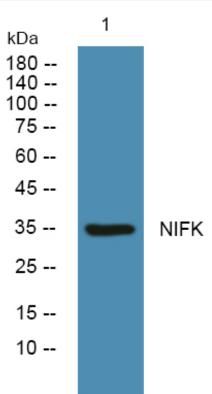
Western blot analysis of lysates from K562 cells, primary antibody was diluted at 1:1000, 4° over night
