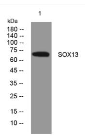
Western blot analysis of lysates from HEK293 cells, primary antibody was diluted at 1:1000, 4° over night
