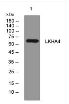
Western blot analysis of lysates from KB cells, primary antibody was diluted at 1:1000, 4° over night
