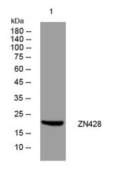
Western blot analysis of lysates from THP-1 cells, primary antibody was diluted at 1:1000, 4° over night
